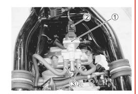
• Disconnect the vacuum hoses ④ from each throttle body.
