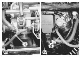
• Connect the respective vacuum tester hoses to ⑤ each nipple on the throttle body.
