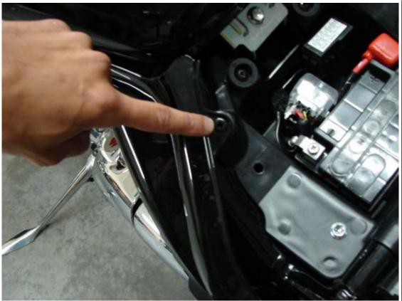
Using a small screwdriver, push in the center of this pin and remove it. Gently push the body panel forward to release the front from the front slide clip, now pull out on the body panel. There are two anchors mounted in rubber toward the rear of this panel, they will pop out by simply applying outward pressure. At this point swing the body panel around the rear footpeg and allow to hang from the seat release cable.
