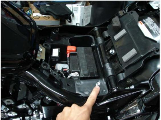
After releasing these bolts the computer and it's mounting cage will be free.
